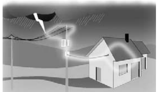
Direct lightning strike on an overhead line
