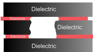
Fig. 4 illustrates "self-healing". The electrode layers in the area where they were short circuiting have been vaporized, thereby eliminating the short circuit.
