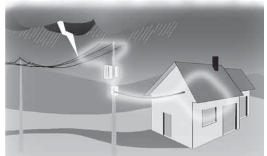
Direct lightning strike on an overhead line
