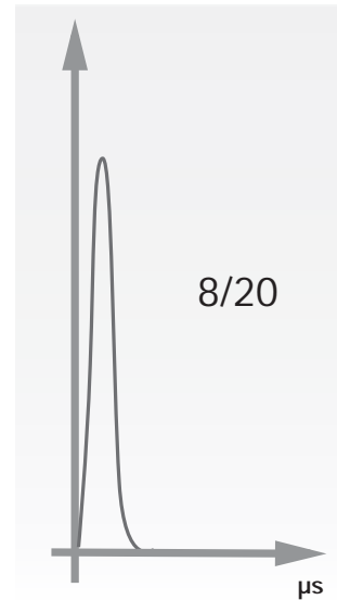
Type 2 Surge Arresters I_{max} : current wave
